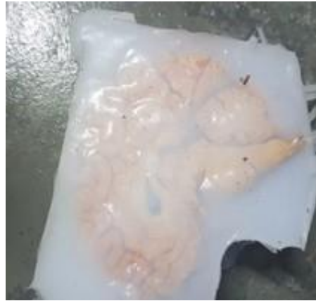
Figure: 1 Brain model in the mold awaiting cure time
