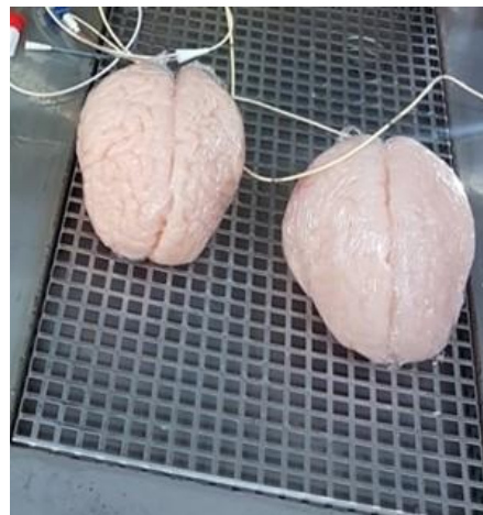
Figure 2: Brain model after being removed from the mold with pia matter
